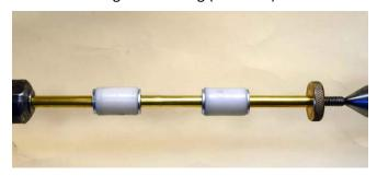
Line up the Duck Call Tooling Kit (BHW 190) on the mandrel as shown -
